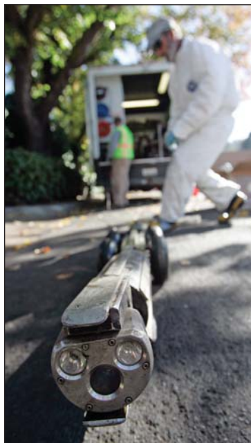
Sal Galindo prepares an Omni Eye-2 camera for a trip through a sewer in Belvedere, Calif. (Photo by Chad Surmick)
